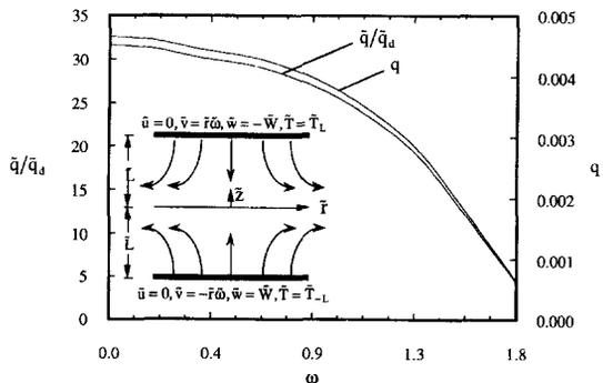
Fig. 1.  $\bar{q}/\bar{q}_d$  and  $q$  vs  $\omega$  ( $Re_L = 600$ ,  $Pr = 1$  and  $\bar{T}_{-L} = 0.8$ ).
