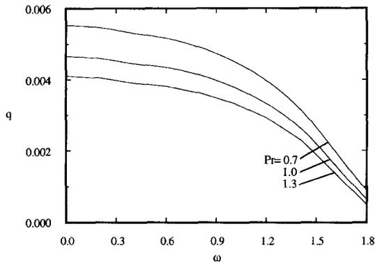
Fig. 2. Efficiency of heat transfer  $q$  vs  $\omega$  for  $Pr = 0.7, 1.0$  and  $1.3$  ( $Re_L = 600$  and  $T_{-L} = 0.8$ ).
