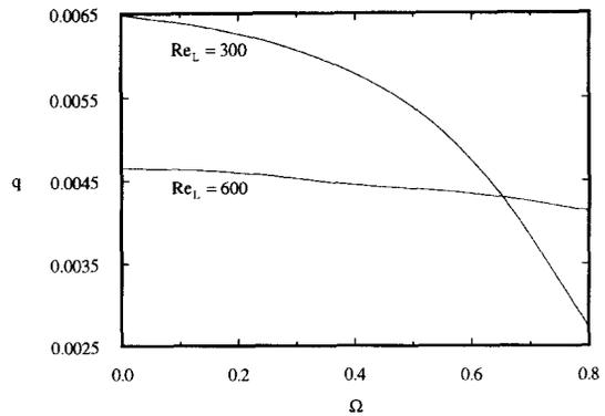
Fig. 3. Efficiency of heat transfer  $q$  vs  $\Omega$  for  $Re_L = 300$  and  $600$  ( $Pr = 1$  and  $T_{-L} = 0.8$ ).
